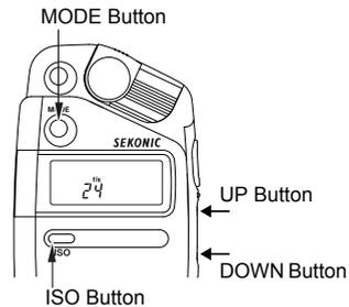
5. Press the **MEASURING** Button to take a measurement. Measurements will be taken continuously and displayed as aperture values as long as the button is pressed. Releasing the **MEASURING** Button will hold and display the last measured value.
