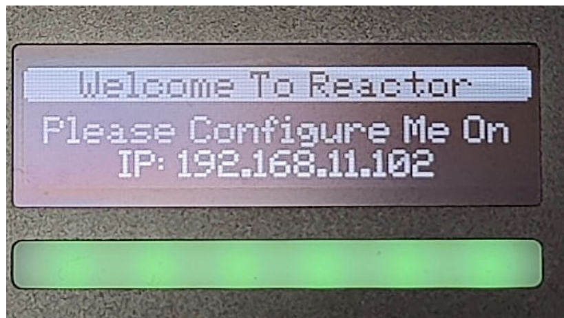
Figure 3: IP address shown for a SKAARHOJ controller.
