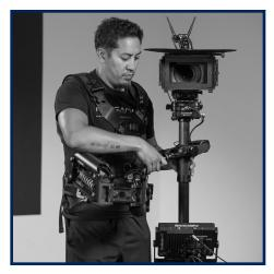
The ROLL dial controls the strength of the motors along the roll axis. Start with low assist and add strength as needed.
