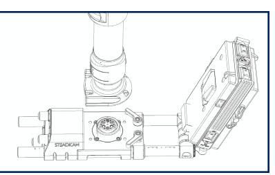
To reinstall the post on the base, align the flat spot on the post connectors. The straight edge of the post foot will align behind the electronics box of the base.
