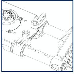
To slide the batteries, unlock the battery rods by rotating both clamp levers perpendicular to the battery rods.
