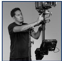
To set the ROLL trim, SHORT-press the trim button on the stage and position the sled to the new level position while the LEDs blink for 5 seconds. When LED blinking stops, your new horizon position will be stored in memory. Set independently for high or low modes
