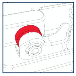
Turn the adjustment wheel to dial in the tension. Turn clockwise to tighten, counterclockwise to loosen. Make small adjustments.
