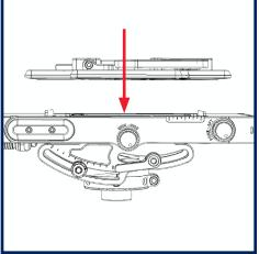
Replace the stage top STRAIGHT down onto the stage. DO NOT slide the top into place, which may damage the VOLT electronics. DO NOT pinch any cables, and ensure internal power cables can slide freely.
