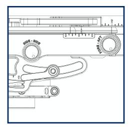
Lock both clamps and re-balance slightly fore-aft.
