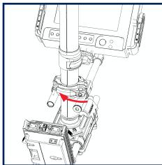
Confirm the marks are lined up with the reference line, so the monitor is square to the rig, and close the clamp lock.
