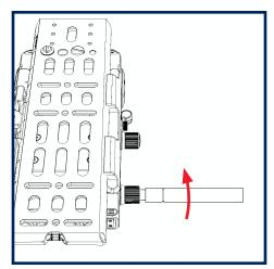
Tighten the nut on the opposite side a small amount as well. Adjust the tension a little at a time and sneak up on the perfect setup.
