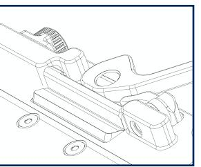
The stage is ready for the camera plate. Note that the dovetail lock and clamp lever are both open.
