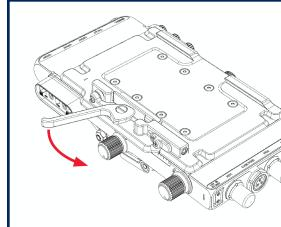
Close the clamp lever so nothing catches on it! To reinstall the dovetail, you'll open the lever and slide the safety latch.
