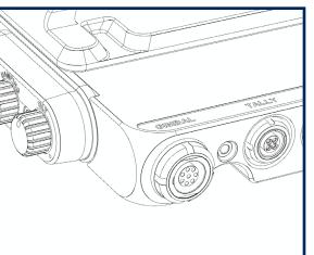
Plug the gimbal cable into the port at the top stage, and wrap a couple loops around the post on its way down to the gimbal.
