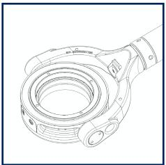
Install the pan bearing lock until finger tight to ensure proper threading, then finish tightening with the Blue Whale tool.
