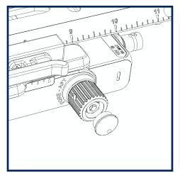
Remove the covers on one PAIR of stage drive knobs. A penknife or fine blade screwdriver works nicely.
