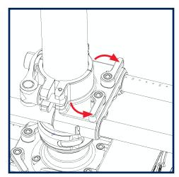
To move the monitor fore and aft on the rods, loosen the clamp levers and slide. Re-lock clamp levers to secure the monitor rods.
