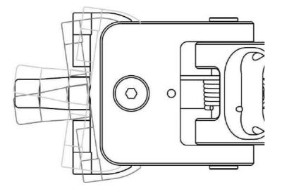
Thanks to two screws on the mating block, you can change the tilt-on angle of your Arm X1. The tilting adjustment is closely related to the operator posture.
