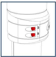
Use a 3/32" Allen wrench to turn each screw an equal, tiny amount. You don't want to over-tighten these, take your time.
