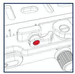
Re-tighten the lock screw before testing the clamp.
