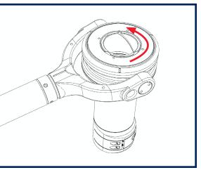
Use the "outside" pins of the Blue Whale tool to loosen the inner ring from the gimbal grip.
