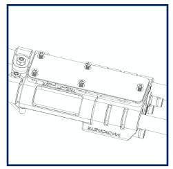
Remove the screws holding on the delrin base cover. You'll use the same screws to attach the dovetail, but set aside the cover.
