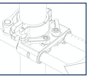
Adjust the clamp locks with the clamp levers closed.
