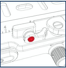
Use a 7/64" Allen wrench to loosen the lock screw approximately one-half turn.
