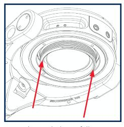
Invert the gimbal, carefully press the inner ring out of the bearing, and set that aside.
