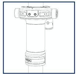
The over-center lock on the gimbal clamp is adjusted while the clamp is closed.
