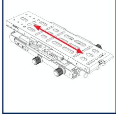
Test to see if the dovetail clamp holds firmly by trying to move the dovetail plate with your hands. Test the clamp lever movement. Repeat adjustment if necessary.
