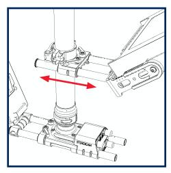
Test the holding power of the rod clamps to ensure the monitor or batteries will not slide when locked.
