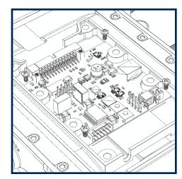
Fasten the Volt brain to the stage chassis with the four included screws, one in each corner.
