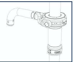
The gimbal remains on the post, and the trunnion screws remain in place. Use the Blue Whale tool to remove both side covers.
