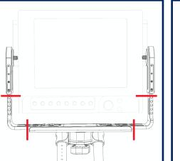
Use the markings to keep the monitor symmetrical side to side and on the uprights. Tighten all of the screws.
