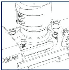
Use a 9/64" Allen wrench to remove the four screws from the post connector.
