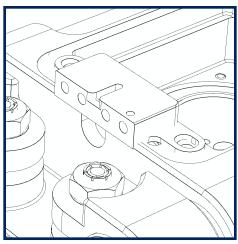
Reposition the pre-wired multi-pin block as shown, so it lines up with the screw holes and the space in the dovetail.
