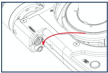
Route the encoder cable over the Volt body, to the side of the gimbal, and connect at the Encoder port.
