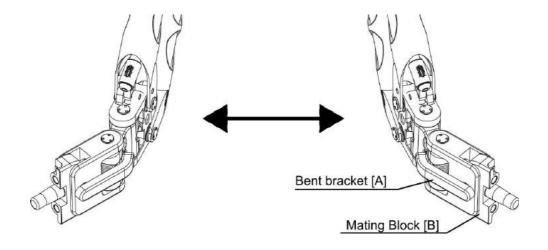
Using the supplied key n.5, loosen the tilt adjustment screws and remove the screw that holds the mating block bolted to the Arm. Remove the bent bracket [A] which preloads the spring in the joint of the mating block. Flip the mating block side [B] and replace back the
