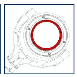
Applying even pressure to both sides, ease the pan bearing out of the gimbal. Never use tools to pry on a bearing!
