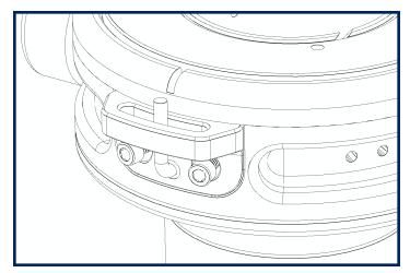
Remove the tiny hex screws from the cover in the gimbal housing, and install the pan encoder in its place with the cable side up. Reuse the same two screws to fasten it.
