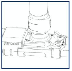
Insert firmly until the post connector sits flush on the base and install the four screws. Tighten with ample torque to secure the post.
