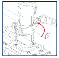
Reposition the monitor mount on the other post, or flip it over for low-mode. Close the clamp around the post or post brake.
