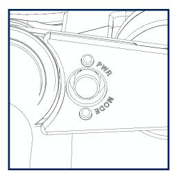
LONG pressing the gimbal thumb button switches operating modes from normal to friction, and back again.
