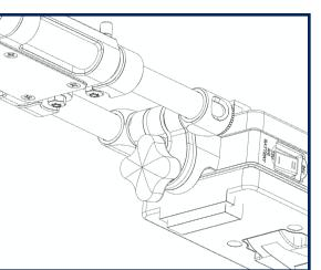
Support the batteries with one hand and loosen the battery clamp knob with the other.
