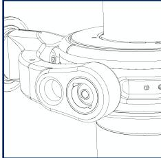
Replace the cover with a thread adapter over the trunnion screw, on the side of the gimbal where you'll mount the motor assembly.
