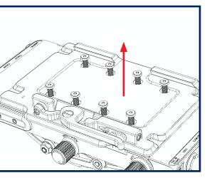
Remove the eight hex screws securing the dovetail clamp to the top stage chassis. Carefully lift the stage top STRAIGHT off.
