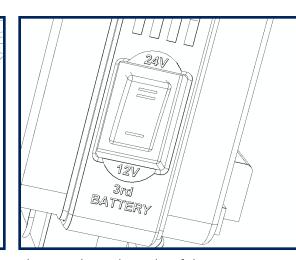
The switch on the side of the main battery mount is now active. Use it to select whether the 3rd battery is wired parallel (12V) or series (24V) with the rear (#1) battery.
