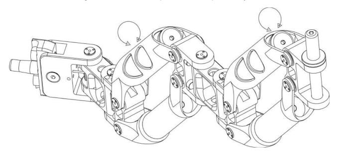
7. Tighten the preload screw until the small plate of the screw itself will be aligned to the first mark in the preload indicator. (as shown in the picture)
