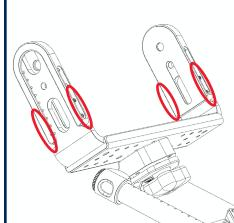
Loosen the eight set screws to adjust the height of the uprights. Fit the monitor height so it clears the yoke when flipped 360°.
