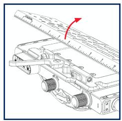
Keeping the safety latch held to the side, tilt the dovetail plate out of the dovetail lock.
