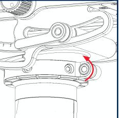
Use a 7/64" Allen wrench to loosen the clamp screw. This just needs to be loose, not removed.
