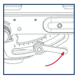
Unlock both tilt lock clamps. There's one on each side of the stage. Open about a half-turn, and tilt the stage as you prefer.
