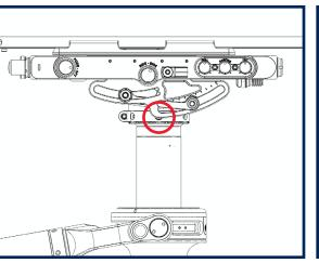
If you have a tilt stage, start with the tilt set slightly upward, which allows access to all screws.
