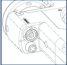
Plug in the cable at the gimbal. Make sure the pan encoder cable is also plugged in next to it.
