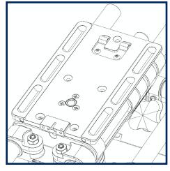
Install the dovetail with the screws. The sled is now ready to accept the battery mount.
