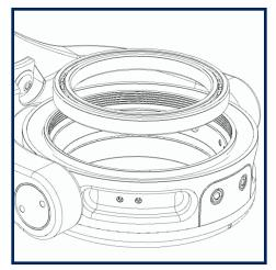
Carefully insert the pan bearing into the outer ring using light finger pressure. When properly aligned, the bearing will easily slip into position. If the bearing binds up while inserting, remove the bearing and start again, being sure to properly align.
