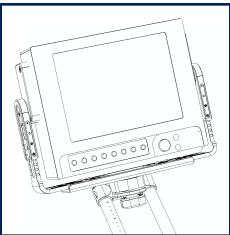
Double check that the monitor is square to the rig, is held securely in the yoke, and rotates smoothly.
