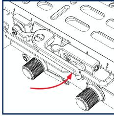
Close the clamp lever to firmly secure the dovetail and camera to the stage.
