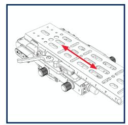
The camera and plate can be moved fore and aft for coarse balancing, but the safety stops prevent it from sliding off.
