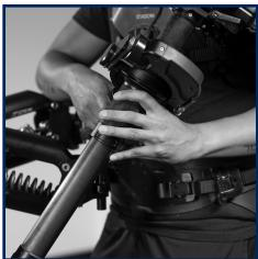
Damping works like friction to keep the sled from oscillating. Use as little as possible, in proportion to your TILT strength.
