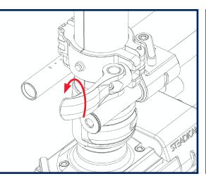
Open the clamp lever, and then turn the lever counter clockwise about 10 turns until it clears the swing arm.
