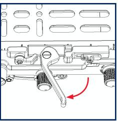
Open the clamp lever. The dovetail is still retained by the safety latch.
