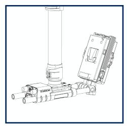
To remove the base, start by removing the monitor mount to make it easy to access the screws.
