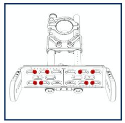
Loosen these eight hex screws to adjust the width. You may need to re-arrange the screws in different threaded holes, but use all eight.
