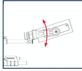
loosen the pivot clamp knob and rotate the yoke around the monitor pivot.
