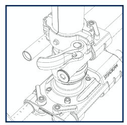
To move the mount on the post, support the monitor and flip open the clamp lever.
