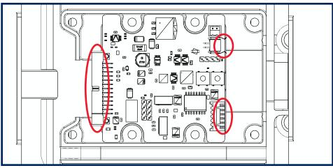
Inside, you'll find three cable sets with connectors that attach to the Volt circuit board, the largest is at the front of the stage. Align the circuit board as shown, and plug them in. Make sure each connector is orientated properly, and be gentle!
