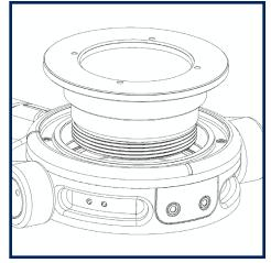
Slide the inner ring into the pan bearing. If aligned properly, the inner ring should slip into position with very light pressure.
