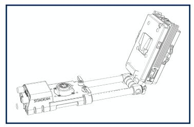
Slide the batteries to either balance the rig or move to your preferred position. Then re-lock the clamp levers before checking drop time.
