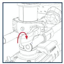
Close the clamp lever around the clamp, and twist the lever about 10 turns back in, setting the clamp tension you prefer.
