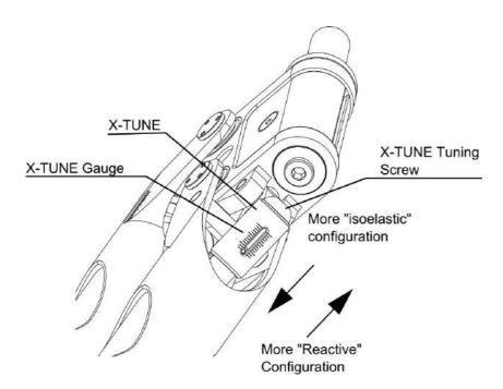
The SmartSystem Arm X1 is equipped with an exclusive tuning system called X-TUNE. It let to change the dynamic behaviour of the Arm itself.
