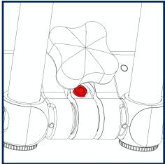
Use a 7/64" Allen wrench to either tighten or loosen the brake screw to achieve the desired amount of friction to support your setup.
