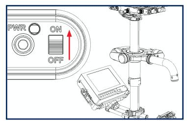
Align the gimbal handle along the REAR of the post, and simultaneously power on the Volt.
