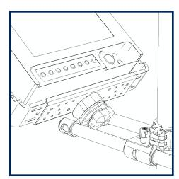
Adjust the friction hinge with the clamp knob loose. This allows you to feel the effects of your changes.
