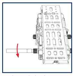
Use the supplied tool (815-7971) to hand-tighten one nut a small amount.
