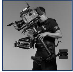
Hold the sled at your desired tilt angle, and short press the button. The new trim is memorized immediately. This can be done on the fly, even during a shot, a huge benefit to your operating.
