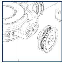
The trunnion pulley threads onto the opposite side, no thread adapter necessary. Use the supplied Blue Whale tool to tighten the pulley in place.
