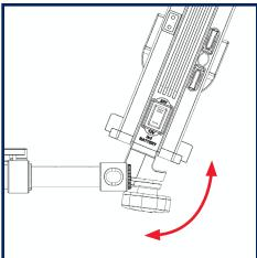
Rotate the batteries to the angle you desire and re-tighten the battery clamp knob.
