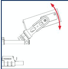
For fine angle adjustment, perhaps To pivot the monitor in an arc, to reduce glare, just tilt the monitor by hand. No fasteners required.
