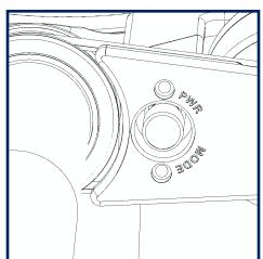
SHORT pressing the gimbal thumb button creates a tilt trim in normal mode.
