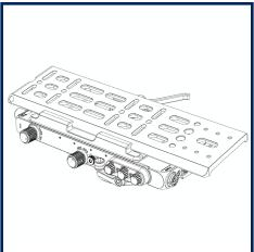
Place the dovetail against the passive side of the clamp, and tilt the plate into the dovetail lock.
