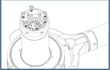
If you need access to the gimbal, remove the six stage connector screws and separate the connector from the top of the post. Your gimbal is now free to slide off for maintenance or to share with a friend!
