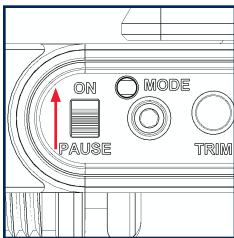
When the rig is up, and you're ready to go, run the Volt by switching the pause switch to ON.
