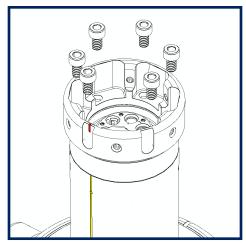
Align the stage connector's red mark with the post reference line, and carefully press into place. Tighten each screw a little bit, in a criss-cross pattern, until all
