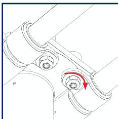
Turn each locknut a small amount with an 11/32" wrench. Test that the clamp levers open and close smoothly.
