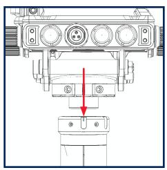
Align the center of the stage with the red line on the post connector. Press firmly until the stainless ring is flush.
