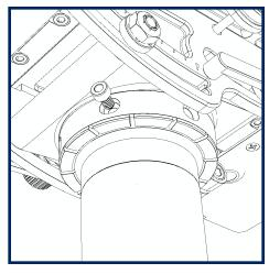
Use a the same Allen wrench to remove the six screws from the post connector.
