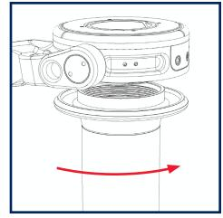
Hold on to the inner ring and screw on the gimbal grip until it's fully seated.
