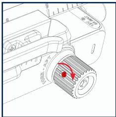
Re-tighten both locking set screws before testing the drive knobs.
