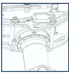
Install the six screws with a 7/64" Allen wrench. Tighten with ample torque to secure the stage.
