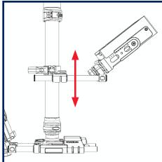
Slide to the desired height, and align the mark on the post clamp with the reference line to ensure the monitor is square to the rig.
