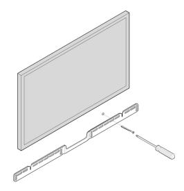
Screw the 2 knobs into the back of the soundbar until they are fully tightened.
