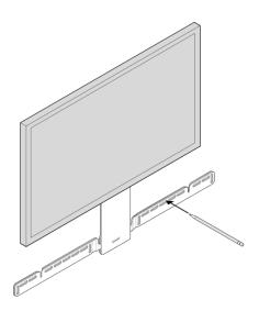
If you're using the included wall anchors, use a 5/16" drill bit to drill the pilot holes and then insert the wall anchors. Don't use the anchors if you're drilling into wood or plastic.
