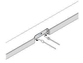
Slide the soundbar down so the knobs fit into the slots on the wall bracket. Make sure the touch controls are facing up and the soundbar is fully seated.
