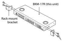
Rack mount bracket attachment screws
