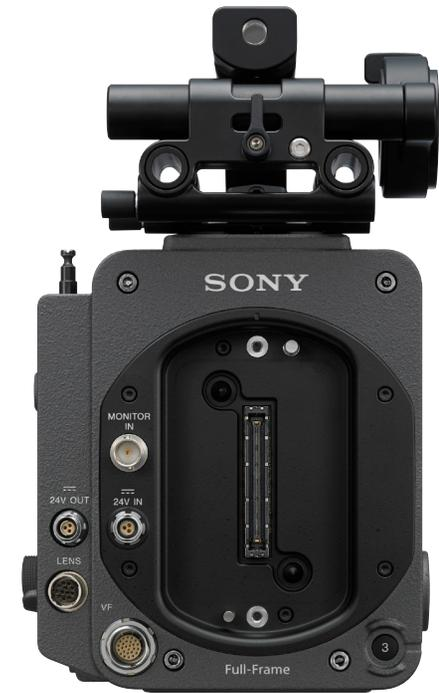
The VENICE camera body plate has a 24V DC input connector (Fischer 3pin). This makes it possible to provide 24V DC output at the camera head using a Fischer 3pin cable. When 12V DC output is required, the Hirose 4pin connector on the VENICE camera can be utilized by using Hirose 4pin to Fischer 3pin cable.
