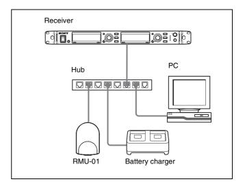
Use straight LAN cables to connect the receivers, RMU-01, battery chargers, and computer via a hub. When the network connection is correctly made, the LED on the LAN connector area at the rear of the receiver lights up green.
