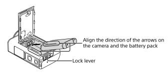
Close the cover securely, then slide the lock lever up to
