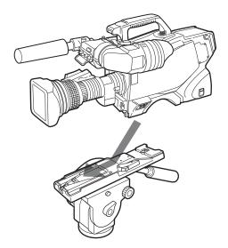
3 Make sure that the camera is securely attached by moving it back and forth.
