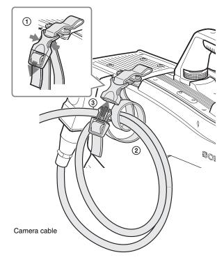
5 Adjust the length by pulling down the end of the belt.
