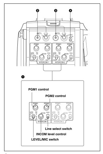
**1** INTERCOM1 and INTERCOM2 controls and switches There are PGM1 and 2 controls incorporated with a line select switch, a LEVEL/MIC switch, and INCOM level control each for intercom line 1 and 2.
