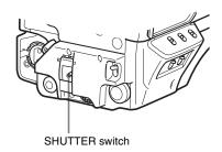
The current shutter setting will be displayed in the setting change/adjustment progress message display area of the viewfinder screen for about three seconds.
