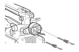
Using the two bolts (M4  $\times$  8) and the washers removed from the camera in step 2, attach the rotation mechanism assembly of the BKW-401 to the camera.
