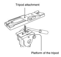
Place the camera on the tripod attachment, and slide forward it along the groove of the tripod attachment until it clicks.
