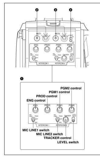
● INTERCOM1 and INTERCOM2 controls and switches The reception level controls are common to intercom 1 and intercom 2. The talk lines can be set independently for intercom 1 and intercom 2.
