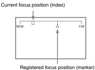
You can set the focus to the registered point easily by adjusting the focus until the index position overlaps the marker position (adjusted state). In the adjusted state, you can display a color frame and marker name on the viewfinder screen.
