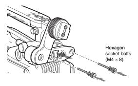
Adjust the front-rear position so that the camera handle does not interfere when you rotate the BKW-401 arm upwards.
