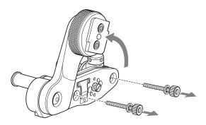
2 In the same manner as step 1, remove the viewfinder shoe of the camera from the front-rear positioning mechanism.
