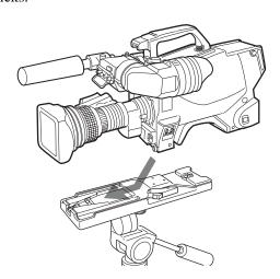
**3** Make sure that the camera is securely attached by moving it back and forth.
