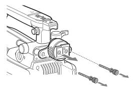
**3** Using the two bolts  $(M4 \times 8)$  and the washers removed from the camera in step **2**, attach the rotation mechanism assembly of the BKW-401 to the camera.
