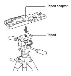
**2** Place the camera on the tripod adaptor, and slide forward it along the groove of the tripod adaptor until it clicks.
