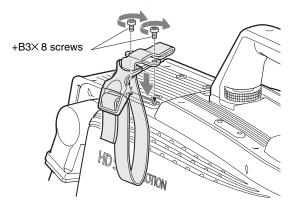
4 ① Release the buckle, ② bundle the cable with the belt, ③ then lock the buckle again.
