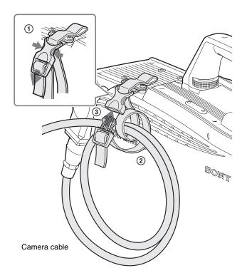
**5** Adjust the length by pulling down the end of the belt.
