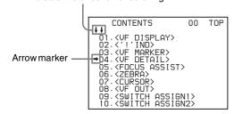
Rotate the MENU SEL knob/ENTER button to align the arrow marker (→) with the desired page indication, then push on the MENU SEL knob/ENTER button.
