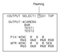
Turn the CONTROL knob to change the displayed page to the desired page, then press the CONTROL knob.
