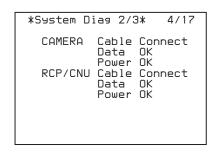
CAMERA Cable: Camera cable connection status CAMERA Data: Camera data transmission status CAMERA Power: Camera power supply status
