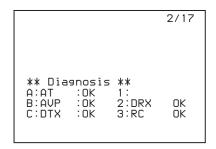
The name of the board connected to the unit's front panel and that board's self-diagnostic results are displayed.
