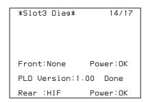
The setting status of the board installed in Slot3 (front/rear) is displayed.
