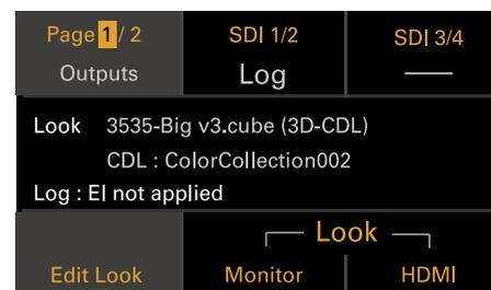
The LUT selection screen has two pages, and you can switch the page by pressing ITEM key 1.
