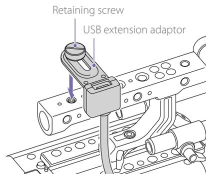
You can adjust the position of the USB extension adaptor over the range shown in the following diagram.
