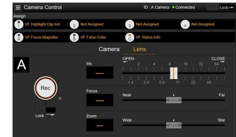
Lens controls for zoom, focus, and iris are displayed on the Lens screen.
