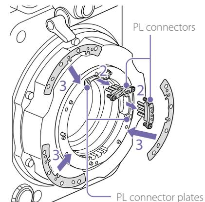
**When using 1/3 arc shims**
