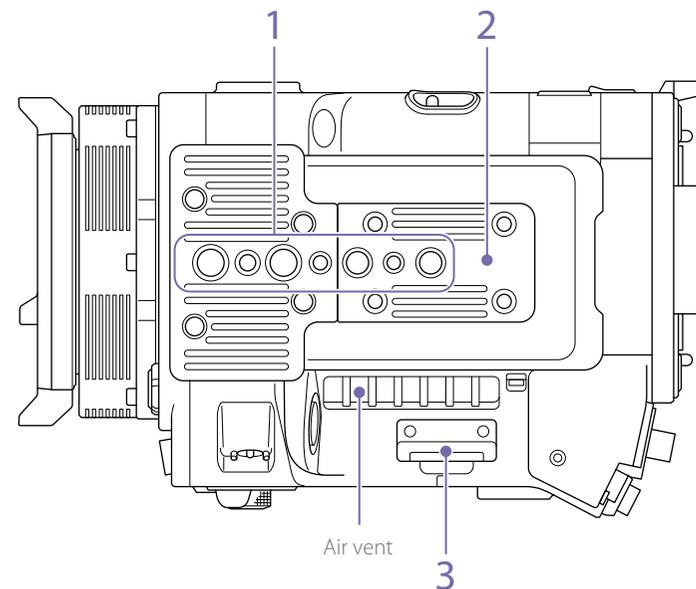
**1. Tripod plate attachment holes**
