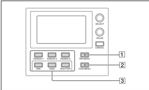
One of the three menus (RM menu, camera menu, or FUNCTION menu) is always selected. When the RM menu or FUNCTION menu is selected, the menu items and settings are displayed on the LCD panel. When the camera menu is selected, nothing is displayed on the LCD panel.
