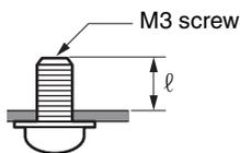
$l$  (contact surface to end of thread) = 6 mm to 10 mm
