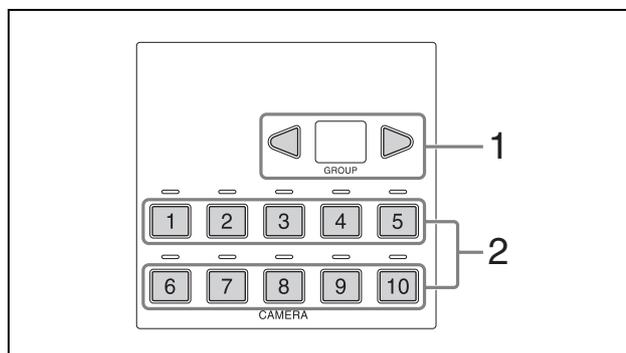
The number of camera numbers that can be assigned to control varies depending on the use of LAN connection or serial connection. The method of selecting the camera number also is different.
