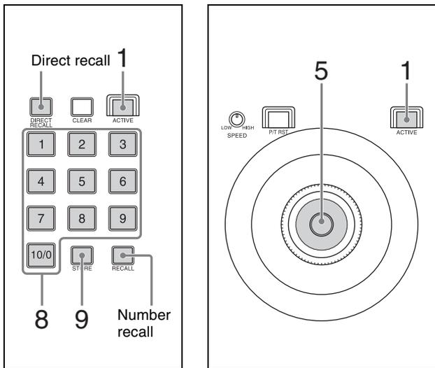
**1 Press the ACTIVE buttons, turning them on (buttons are lit), on the joystick control block and preset memory control block.**
