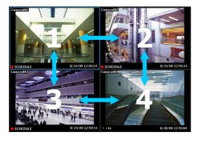
The light blue frame moves to the selected monitor frame, and the selected monitor frame number appears in the screen on the LCD.
