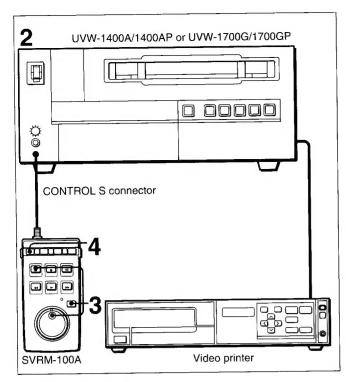
2 Set the output timing on the UVW-1400A/ 1400AP/1700G/1700GP, depending on the type of printer connected.
