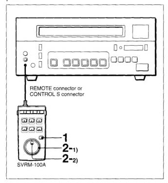
1 Press the JOG/SHUTTLE button to activate jog/shuttle mode.
