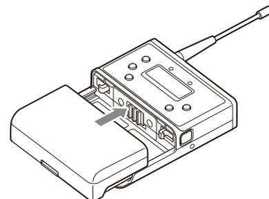
Make sure that the battery compartment is locked securely.
