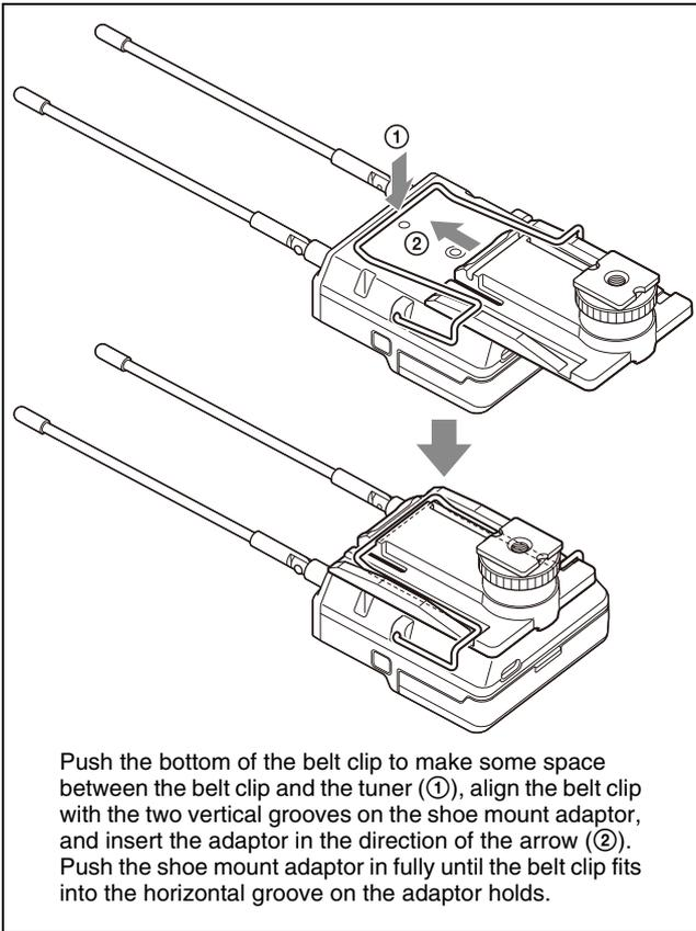
Push the bottom of the belt clip to make some space between the belt clip and the tuner (①), align the belt clip with the two vertical grooves on the shoe mount adaptor, and insert the adaptor in the direction of the arrow (②). Push the shoe mount adaptor in fully until the belt clip fits into the horizontal groove on the adaptor holds.
