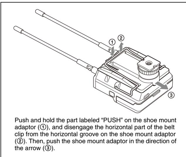
Push and hold the part labeled “PUSH” on the shoe mount adaptor (①), and disengage the horizontal part of the belt clip from the horizontal groove on the shoe mount adaptor (②). Then, push the shoe mount adaptor in the direction of the arrow (③).
