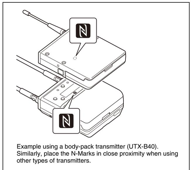
Example using a body-pack transmitter (UTX-B40). Similarly, place the N-Marks in close proximity when using other types of transmitters.
