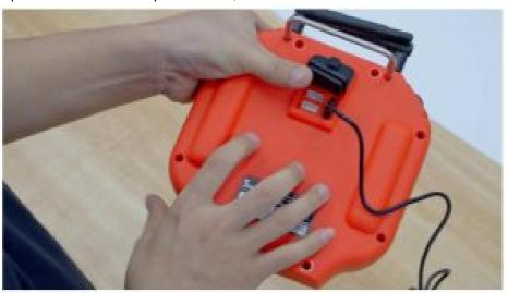
Long press the power button and remain pressing until the update is complete.
