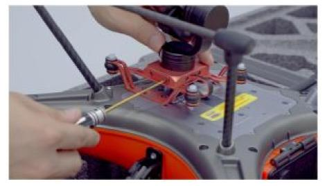
Connect the gimbal to the laptop using the USB cable. Power on the aircraft.
