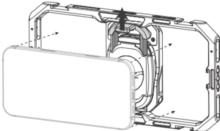
**(5) Phone Clip Adjustment:** To avoid button obstruction and center the phone, use the included Allen wrench to loosen the adjustment screw and slide the clamping column left or right until the phone is centered and the phone clip doesn't cover any buttons.
