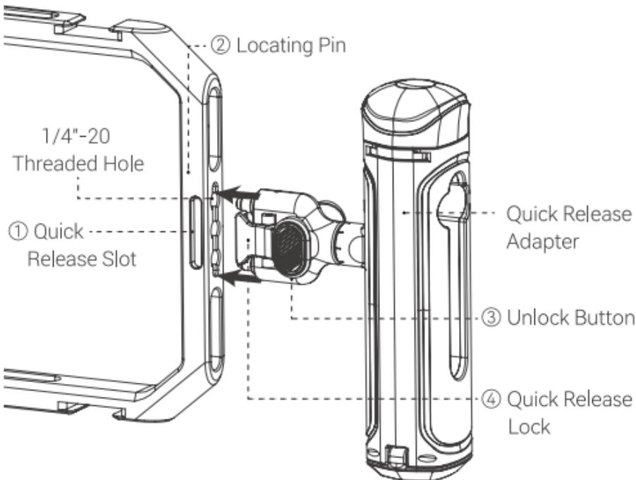
※**Quick Release Unlock:** Press both Unlock Buttons ③ to detach the adapter.
