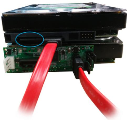
5. Using the remaining included **SATA Cable**, connect the **SATA Host Interface connector** on the **S322SAT3R** to an available **SATA Interface** on your **Computer System**.
