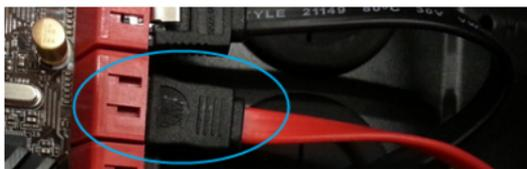
6. Using the included **4-pin to SATA Power Adapter**, connect the **4-pin power connector** on the **S322SAT3R** to an available **SATA Power Source** in your **Computer System**.
