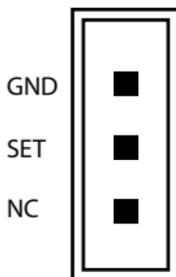
Use the included jumper and the table below, to short the pins and set the mode for your desired configuration.
