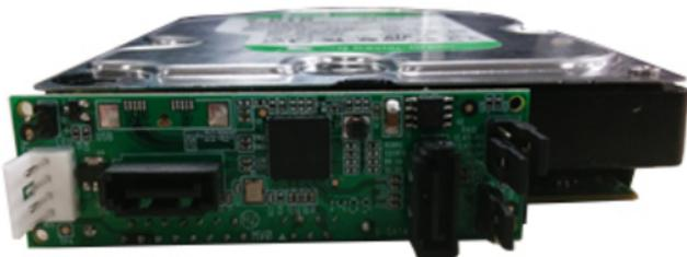
3. Using one of the included **SATA Cables**, connect the **SATA (Data)** connector on the second **HDD/SSD** to the **Drive #2 SATA (DATA) connector** on the **S322SAT3R**.
