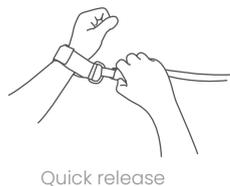
**!** While wearing the safety leash, in order to protect your personal safety in case of emergency, the device can be separated from you by quick release.
