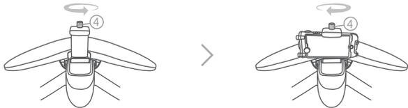
4. According to your shooting needs, rotate the holder to the horizontal or vertical state.
