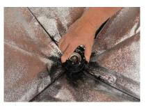
**2**- Center the "O" ring over the bulb socket.
