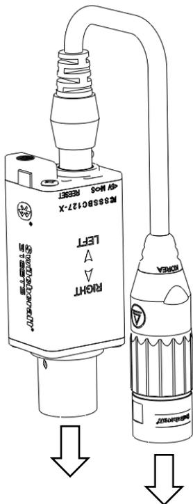
Insert *318BTS* into the audio mixer (Mic level), then connect the audio breakout cable supplied with the unit and insert the other end into a second channel on the audio mixer.
