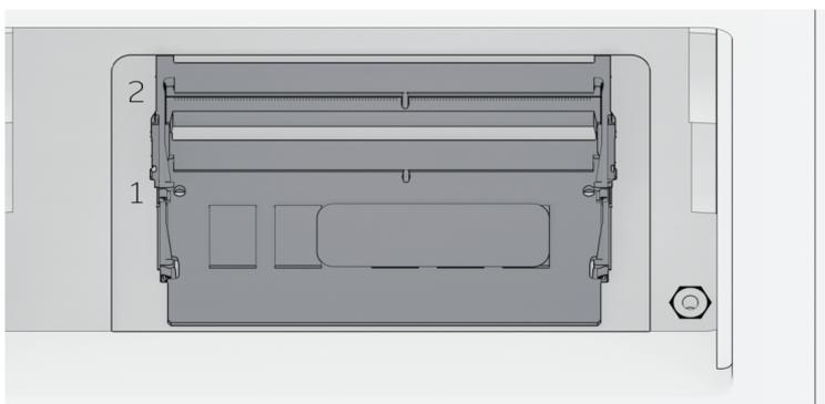
4. Push the levers on both sides of the memory module outward. The memory module will be released from its slot.
