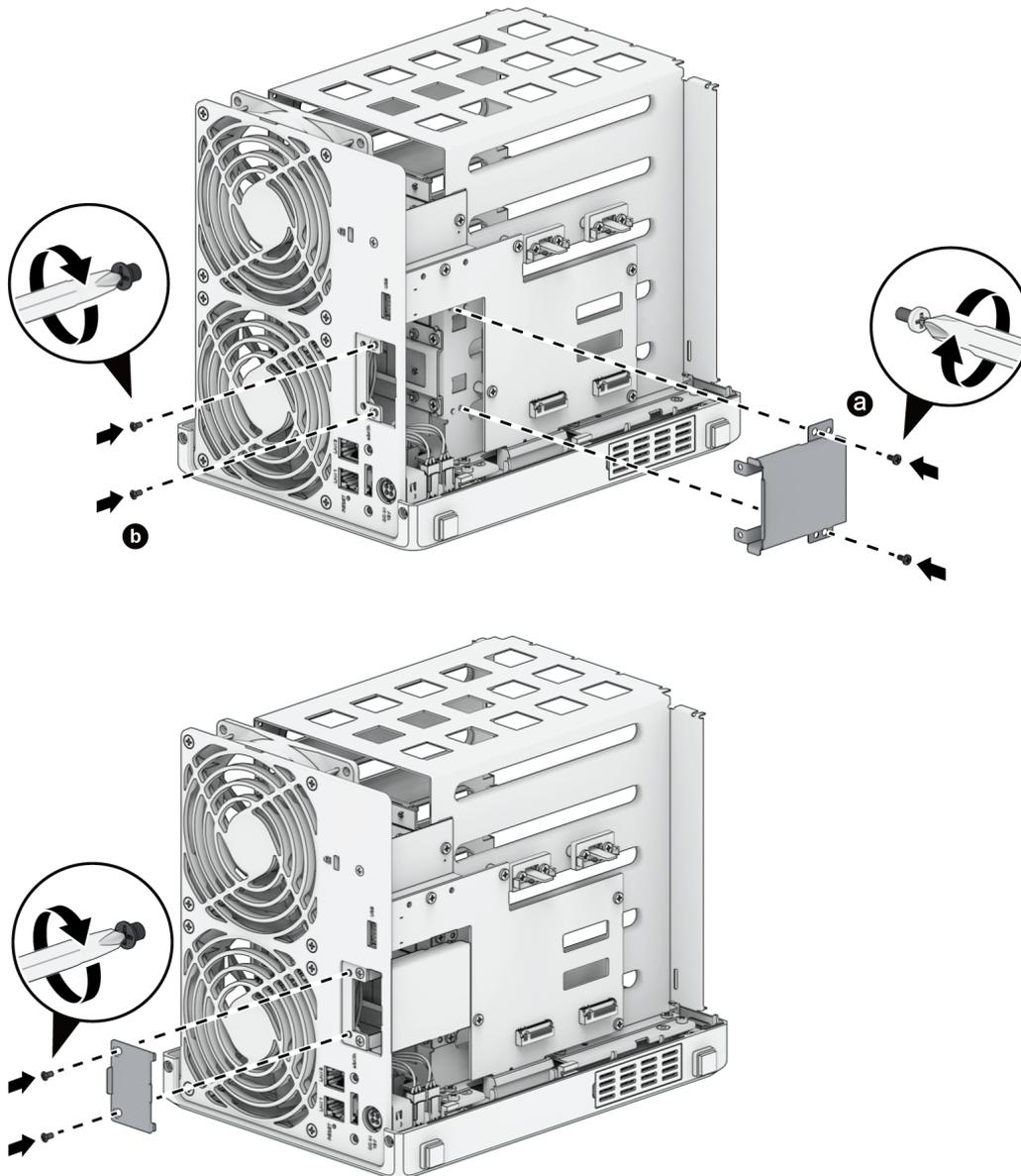
5. Re-install the plastic fan supports and their screws.
