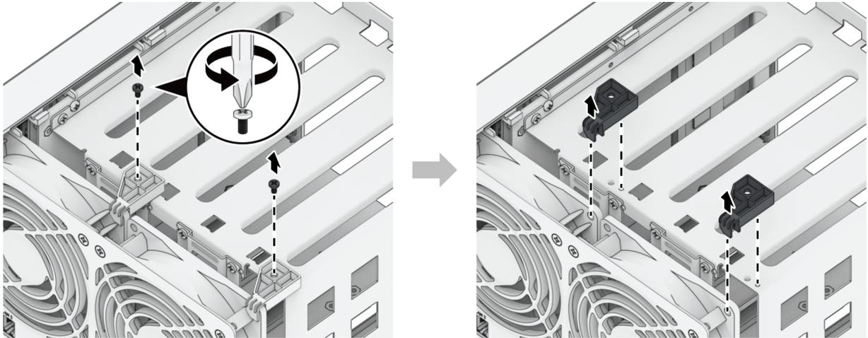
6. Remove the two screws as well as the PCIe expansion shield beneath the fans at the back of your Synology NAS.
