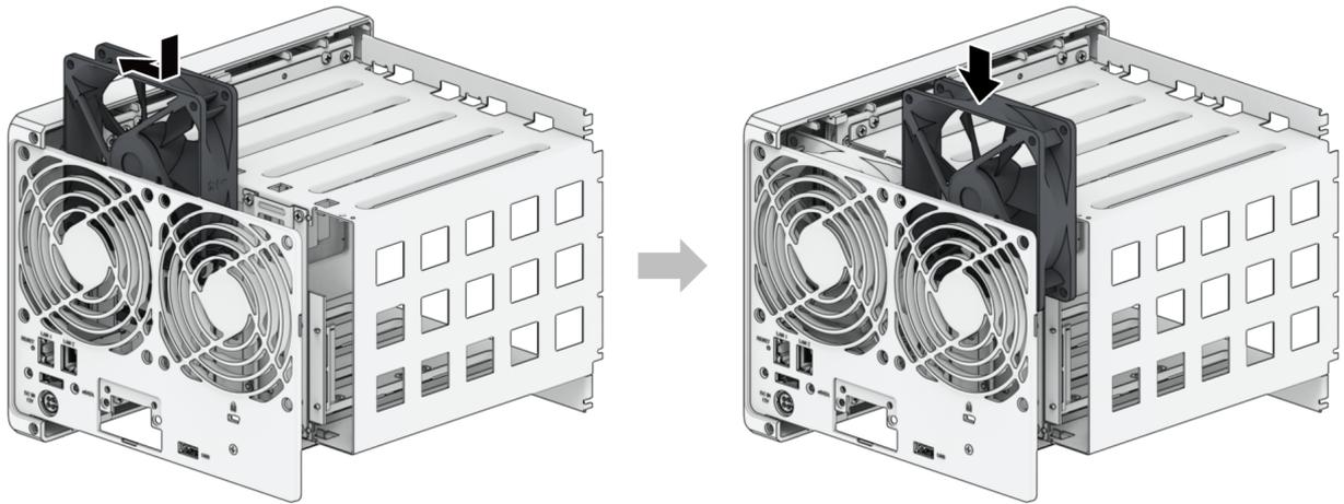
3. Install the backplate screws and connect the fan connectors in their corresponding slot as shown below.
