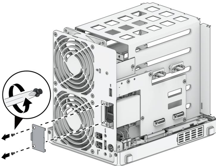
7. Remove the four screws securing the other PCIe expansion shield in place, then the shield.
