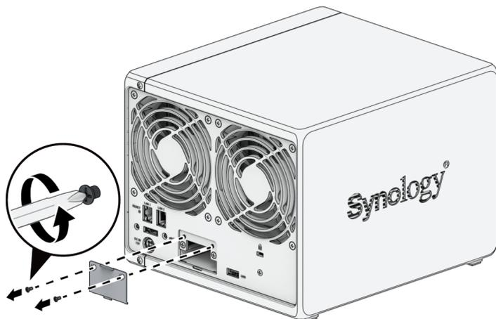
3. Insert the network upgrade module and tighten the two screws to secure the newly inserted module.
