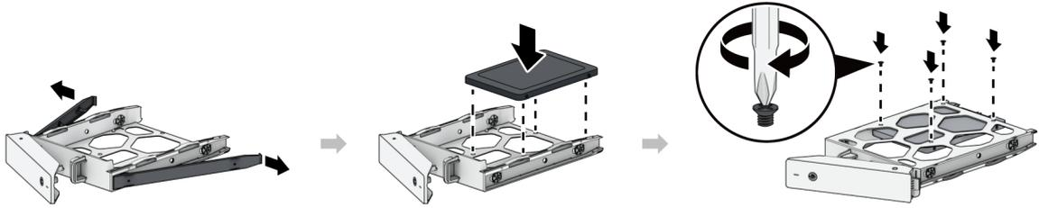
3. Insert the loaded drive tray into the empty drive bay and push it back until you hear a click when the tray is locked into place.
