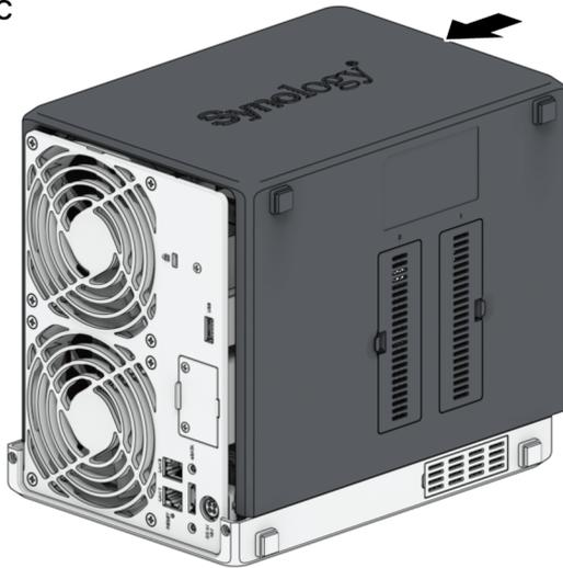
7. Re-install the screws securing the back panel.
