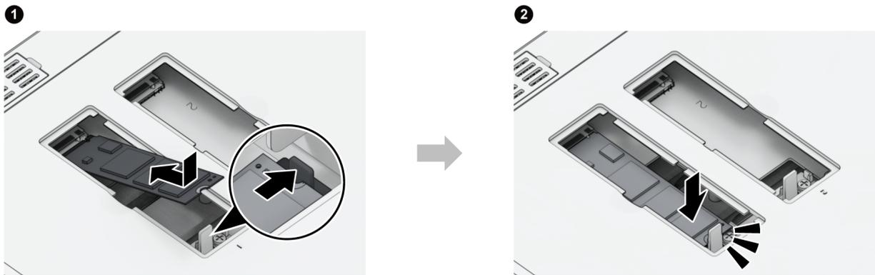
5. If needed, repeat the steps above to install a second SSD module into the second slot.
