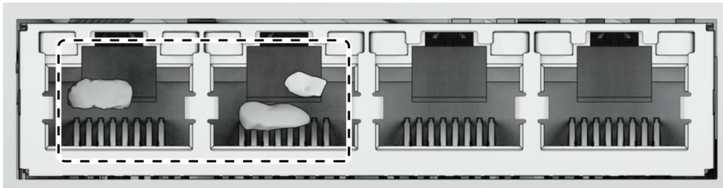
6. Check the interior of the network port for damaged or skewed pins.
