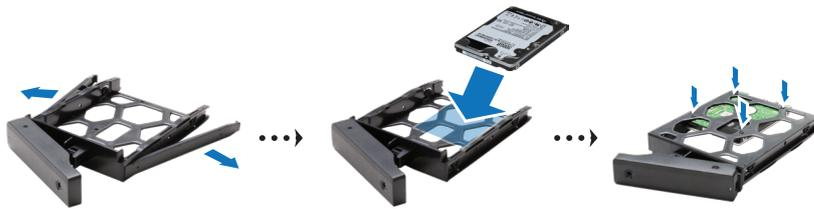
**4** Insert the loaded drive tray into the empty drive bay.
