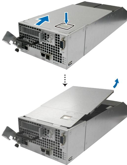
**Note:** When you remove the rear top cover, the sensitive internal components are exposed. Avoid touching anything other than the memory assembly when you remove or add memory.
