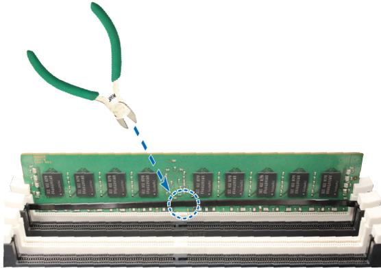
**Note:** Avoid touching any components of the motherboard when you cut the cable tie.
