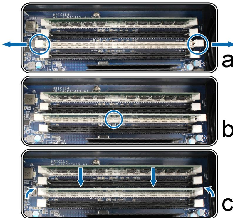
**Note:** Hold the memory module by its edges, and do not touch the gold connectors.
