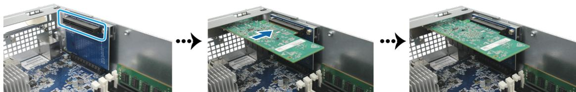
**Note:** Make sure the connector is fully inserted. Otherwise, the network interface card might not be able to function properly.
