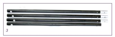
**3.** The crossbar is modular and can be configured to your selected length 3 ways, as in 5′, 7.5′ or a 10′ options. Each tubular section is labeled with a letter. "A" and "D" have a larger hole for coupling to the support stands. "A" mates to "B" to make a 5′ bar, and "B" added to "D" makes a 7.5′ length.
