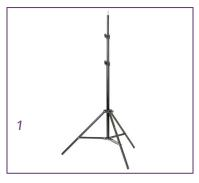
1. Take one of the 6' Support Stands and loosen the knob (lefty/loosey – righty/tighty) that frees the legs. Open the 3 legs to their maximum spread. The 3 spokes that are attached to the center column and legs should be parallel to the ground for the best balance and safety. Raise to center column section to a comfortable height, not fully extended. You will have to connect the crossbar to the tops of the stands and if you start off too high, it will be out of reach.
