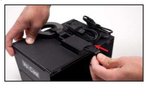
Insert the hook into the webcam module until it clicks into place.
