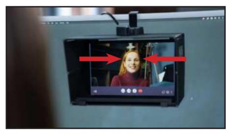
By using a special mirror invisible to the user, the VoxCast's camera is positioned behind the person you are speaking with. The optimum area to look is indicated by the red arrows.
