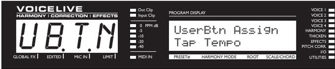
EDIT 1 knob: **USER BUTTON ASSIGN.** Assigns a parameter to be controlled by the USER button. Options include:
