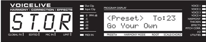
Above is an example of the store screen after editing a preset and pressing store. VoiceLive keeps track of the last thing you changed. Pressing the STORE button again will store the preset to the current location. For example, if the last thing you changed was a Global parameter under the IO and UTIL edit screens, the LCD display would show:
