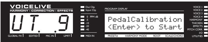
VoiceLive will operate properly with most passive volume and expression pedals. Use this screen to calibrate the pedal. To calibrate the expression pedal follow instructions on the VoiceLive LCD display:
