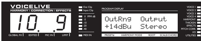
EDIT 1 knob: **OUTPUT RANGE**. This sets the output level range. The value displayed reflects the maximum output level at that setting. Please note that some mixers will produce a distorted signal with a +20dB signal. If you experience distortion and neither the input nor output clip lights are flashing on VoiceLive, try adjusting this parameter to a lower setting.
