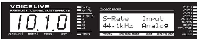
EDIT 1 knob: **SAMPLE RATE**: 44.1kHz, 48kHz or External.
