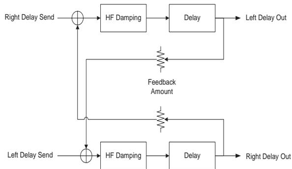
EDIT 2 knob: **DELAY FEEDBACK AMOUNT.** Increasing this value causes the delayed signal to take longer to fade out.
