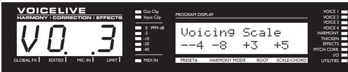
This screen is used to set the voicing of the four harmony voices. Voicing means setting the harmony voice note/pitch with respect to the lead note/pitch. This parameter means different things for different harmony modes. The harmony mode of the preset is shown on the LCD display.
