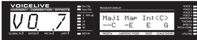
**CUSTOM VOICE MAPPING** (Scale Mode Only). Scale mode harmonies are basically pitch maps. For each input note in a scale you can define a resulting harmony note. VoiceLive has 3 major and 3 minor scale pitch maps for all scale roots, and intervals. The Custom voicing feature allows you to create your own pitch maps. For example, you could define a pitch map so that a C input produces an E output and a D input produces an A output. A good way to work with custom voicing is as follows:
