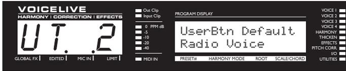
This screen sets the default USER button function. In the preset if the USER button is set to default, then the USER button assignment will come from this screen.
