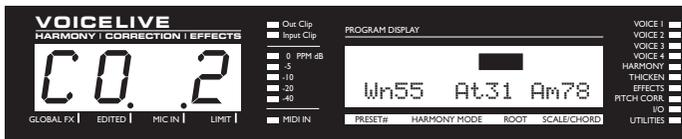
This screen gives access to parameters that determine how subtle or aggressive the pitch correction. The upper line of the display shows in real-time the pitch correction being applied by VoiceLive. The maximum correction displayed is +/- 200 Cents (there are 100 cents per semitone).
