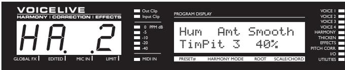
EDIT 1 knob: **HUMANIZATION STYLE**. This is a list of humanization style types. Each Style is made up from a combination of Flextime™ based time randomization, pitch randomization and pitch inflection (scoop). Available styles include:
