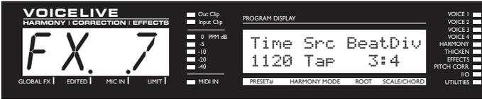
EDIT 1 knob: **DELAY TIME (ms)**. This can be used to manually set a delay time or adjust a delay time entered through tap tempo.
