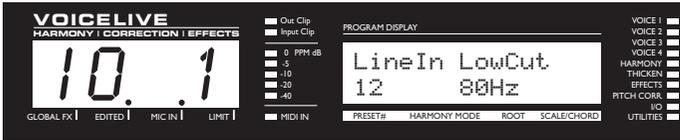
EDIT 1 knob: **LINE INPUT GAIN.** Sets the input gain for the line input.
