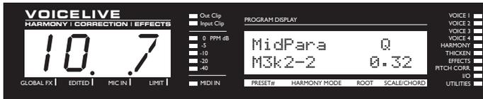
This screen provides control of the fully parametric mid EQ.
