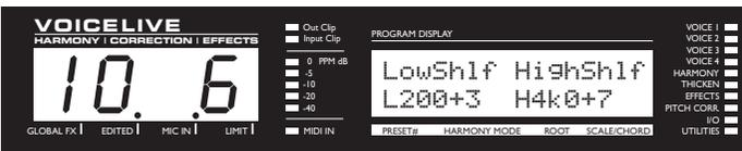
VoiceLive has an extremely flexible 3 band EQ with frequency adjustable high and low shelving bands and a fully parametric band with Q, frequency and Gain controls. This screen gives control over the high and low shelf EQ parameters.
