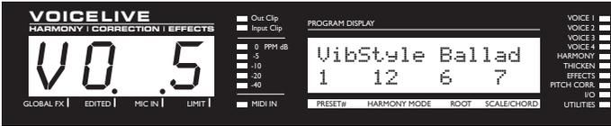
This screen is used to select a vibrato style for each harmony voice. The vibrato styles are based on the analysis of real singers. When changing the style number, the corresponding style description is displayed on the screen. Available Vibrato styles include:
