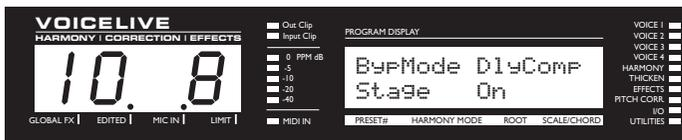
EDIT 1 knob: **BYPASS MODE**. This sets how VoiceLive operates in Bypass as controlled by the footswitches. The Stage setting disables all effect processing except for EQ and Dynamics processing. The Studio setting removes all effect processing including the EQ and Dynamics and outputs the lead signal at full level to the digital output.
