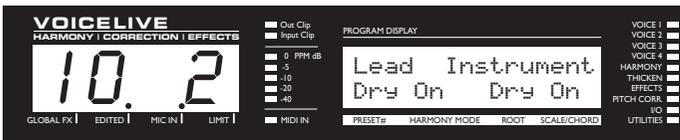
EDIT 1 knob: **DRY LEAD ON/OFF.** Setting this to off removes the dry lead audio from the signal path. This is useful when using the signal from the Mic Pass Thru connector for the dry lead signal or when you want 100% wet output.
