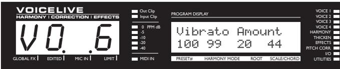
This screen is used adjust the amount of vibrato applied to each voice.
