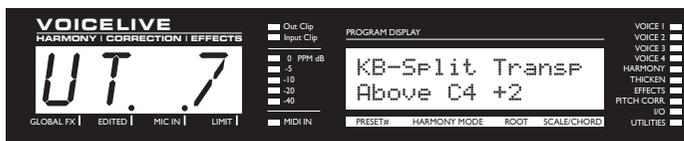
The parameters on this screen allow keyboard players to specify a range of the keyboard to control Notes and Chord mode harmonies. For example using a combination of the three controls below, a user can set the top octave of the keyboard to play notes mode harmonies.
