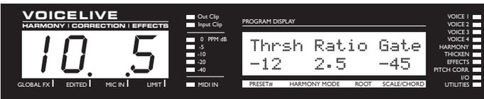
Compressor / Gate settings. The compressor in VoiceLive has auto makeup gain to a maximum of +20dB. This means that the volume level of the signal will be increased for most volume levels of input with the compressor enabled.
