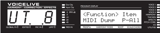
In this screen the selection from the first knob affects the options in the second knob. Once you have made the selections you must press the DATA WHEEL for ENTER to perform the function.
