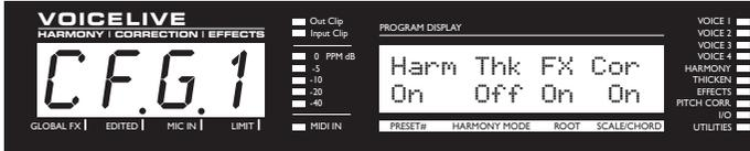
These parameters allow enabling/disabling of Harmony, Thickening, Effects and Pitch correction audio components. The **Voices and Effects LEDs** will reflect the settings of this page.
