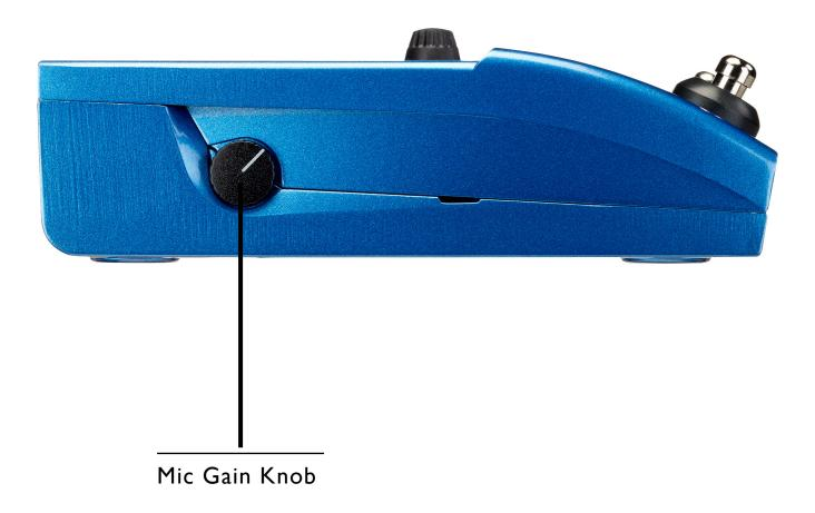
Once you've connected your microphone and selected the Mic Type (pg. 12, Dynamic, Condenser, MP-75), use the Mic Gain Knob to set the input level for your microphone.
