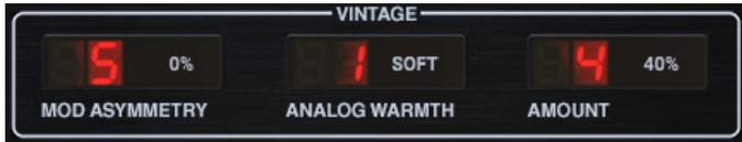
The MODULATION ASYMMETRY parameter was not included in the original TC1210. At 0% setting (5), the modulation waveform is modeled tightly against the original TC1210. The original waveform was carefully designed and is rather complex by nature.
