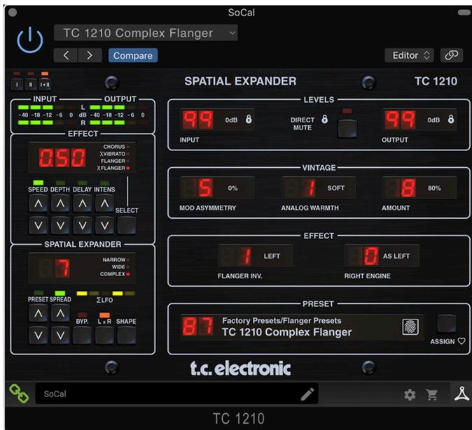
The plug-in is divided into two sections, which are both visible when the “I+II” button at the top left is selected. The left section is identical to the hardware unit and could be considered Primary parameters. These include common items such as depth, delay, and intensity.
