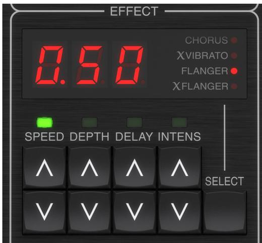
Press the SELECT button to rotate through the 4 effect styles. The red dot will indicate the current selection.
