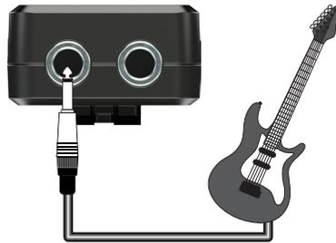
**4** Connect an amplifier to the amp output via an instrument cable with a 1/4" TS connector.
