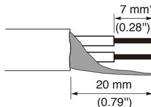
\* Expose 8 mm (0.31") or more when using the above ferrule terminal, and cut off an extra conductor protruding from the sleeve.
