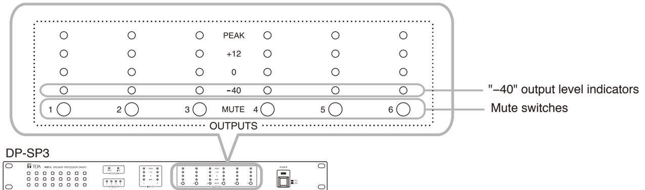
There is a priority order for the mute operating indications between the operation performed from the DP-SP3 and that performed using the DP-SP3 PC Software. If multiple mute operations overlap, then the mute operating indication with the higher priority is activated.
