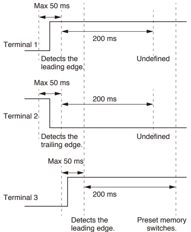
To switch the Preset memory, maintain the given state for 250 ms or more after placing each terminal in the state corresponding to the Preset memory to be recalled.
