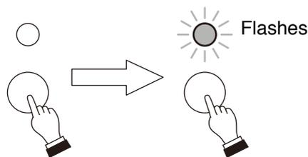
**Step 2.** Press the Mute switch of the corresponding channel, then release it when the “-40” output level indicator of that channel begins to flash.
