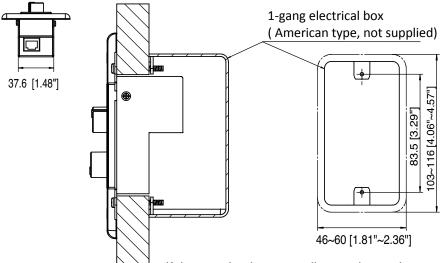
If the opening is too small or too large, the WP-700-AM cannot be mounted in the wall. Be sure to make an opening with dimensions given above when mounting.
