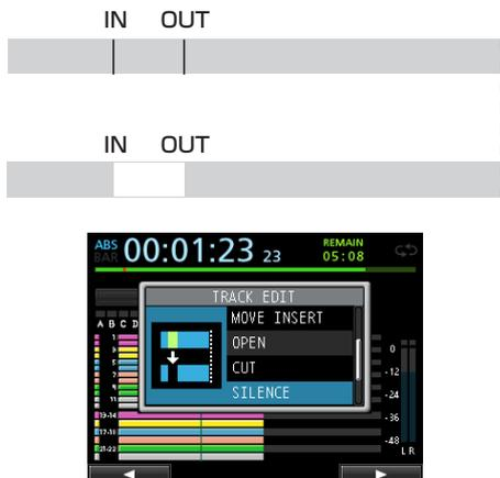
This function cuts (deletes) the audio data between the IN and OUT points on the selected track.
