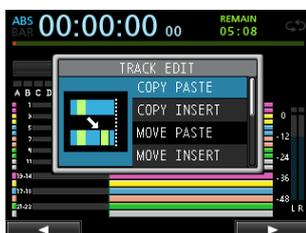
This function copies the audio data from between the IN and OUT points on the COPY source track, and pastes it on the COPY destination track starting from the TO point. This operation does not change the COPY source track.
