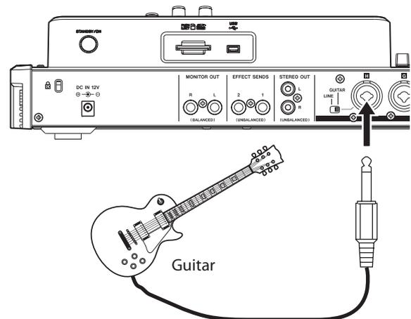
2. Set the **LINE-GUITAR** switch to **GUITAR** on the rear panel.
