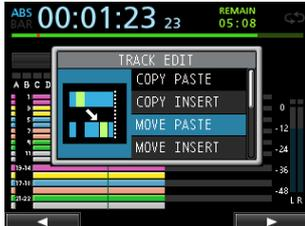
The audio data between the IN and OUT points on the MOVE source track is removed and pasted on the MOVE destination track starting from the TO point. This operation leaves a silence between the IN and OUT points on the MOVE source track.
