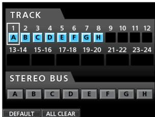
2. Use the **CURSOR** (**▲**/**▼**/**◀**/**▶**) buttons or press the **SELECT** button for TRACK 1 and align the cursor (frame) on the Assign screen with TRACK 1.
