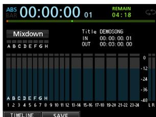
If you play or record, you can hear the signal of the mixed tracks (the signal to be recorded) through headphones or monitoring system.
