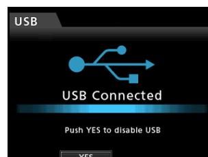
After making a USB connection, you must turn the power on and enable the USB connection in the USB item of the MENU screen.
