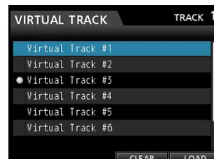
You can also press the **VIRTUAL TRACK** button first, then select a track on the **VIRTUAL TRACK** screen.
