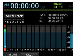
When you raise the fader for TRACK 1, the **STEREO** fader and the **MONITOR LEVEL** knob, you can hear the sound of the guitar through the headphones, and the **L** and **R** level meters move.
