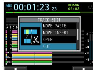
This function cuts (deletes) the audio data between the IN and OUT points on the selected track, and shifts the remaining recording after the OUT point forward to the IN point. Therefore, the track becomes shorter.
