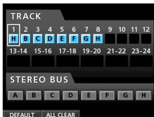
Record the lead guitar sound from INPUT H to TRACK 2. By default, INPUT B is assigned to TRACK 2.
