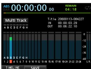
When you raise the fader for TRACK 3, the **STEREO** fader and the **MONITOR LEVEL** knob, you can hear the sound of the mic input through the headphones.
