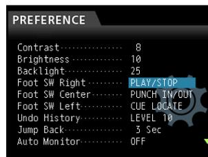
4. Use the **JOG/DATA** dial to select the function that you want to assign to the pedal R (right) of the TASCAM RC-3F foot switch.
