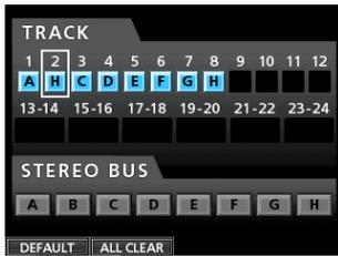
2. Use the **CURSOR** (▲/▼/◀/▶) buttons or press the **SELECT** button for TRACK 3 and align the cursor (frame) on the Assign screen with TRACK 3.
