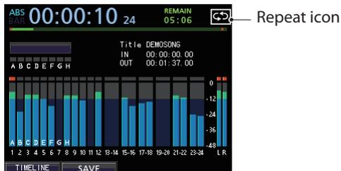
After the playback starts from the IN point and reaches the OUT point, it returns to the IN point and repeats.
