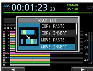
The audio data between the IN and OUT points on the MOVE source track is removed and inserted in the MOVE destination track starting from the TO point. This operation leaves a silence between the IN and OUT points on the MOVE source track.
