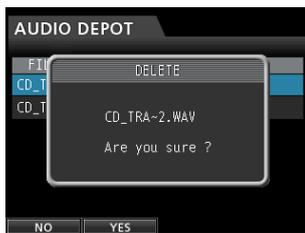
3. Press the **F2** (YES) button to execute the deletion. When you want to delete multiple files, repeat the procedure above.
