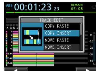
This function copies the audio data from between the IN and OUT points on the COPY source track, and inserts it on the COPY destination track starting from the TO point. This operation does not change the COPY source track.
