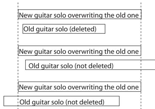
As shown in the illustration, if old audio data is not completely overwritten by new audio data, old audio data cannot be deleted.
