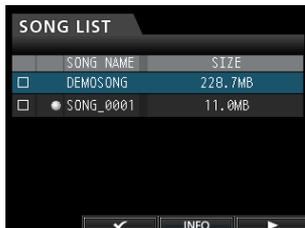
3. Press the **F4** (▶) button to open the sub-menu and then use the **JOG/DATA** dial or the **CURSOR** (▲/▼) buttons to select **CREATE**.
