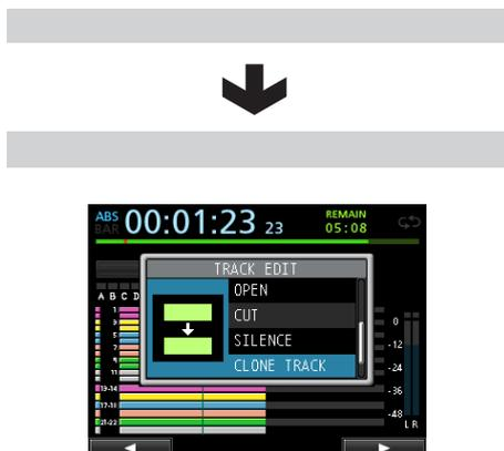
Use this function to duplicate a single track or a stereo track to a different track.
