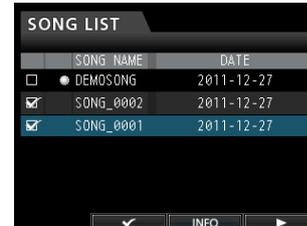
4. Next, press the **F4 (▶)** button to open the corresponding sub-menu. Use the **JOG/DATA** dial or the **CURSOR** (**▲/▼**) buttons to select the item **NAME EDIT** from the sub-menu, and then press the **F4 (▶)** button.
