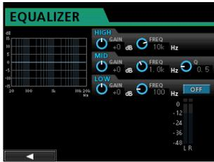
2. Turn the EQ HIGH knob to the left to lower the GAIN knob for HIGH shown on the screen. Set to "-2 dB". This reduces the high frequencies.
