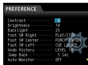
3. Use the **CURSOR** (▲/▼) buttons to select the items you want to adjust such as **Contrast**, **Brightness** and **Backlight**, and then use the **JOG/DATA** dial to make the adjustments.
