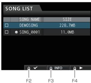
"✓" above the **F2** button shows that "✓" is assigned to the **F2** button when using this screen.
