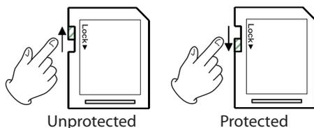
When the protect switch is in the LOCK position, files cannot be recorded or edited on the card. Slide the switch away from the LOCK position if you want to record, erase or otherwise change files on a card.
