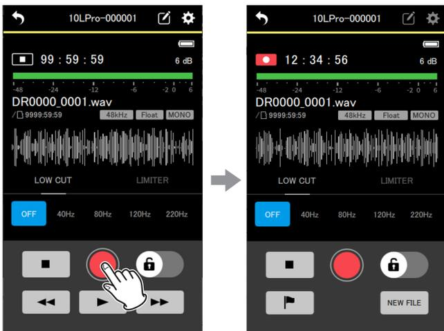
This starts recording with the unit being shown.
