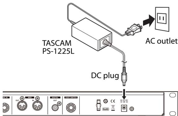
Use the hook (cord holder) on the rear panel to secure the AC adaptor cord. When connecting the cord to the unit, wrap it through the holder to prevent it from becoming disconnected during use.
