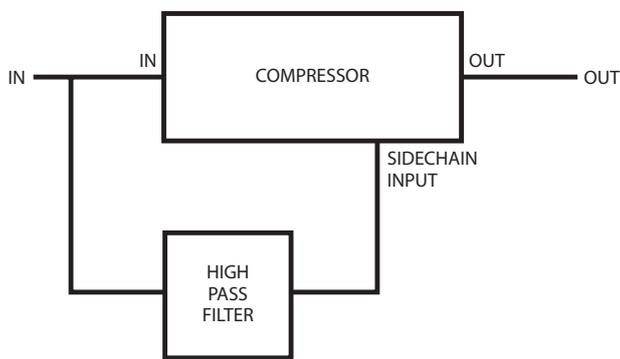
Only the sibilants pass through the highpass filter. When the input signal contains sibilant material, the output of the filter causes the compressor to compress the signal. The compressor only operates when a sibilant is present. The TA-1VP uses a digital algorithm to implement the de-esser function. While the details of the algorithm are quite complex, the resulting effect is functionally equivalent to the diagram above.
