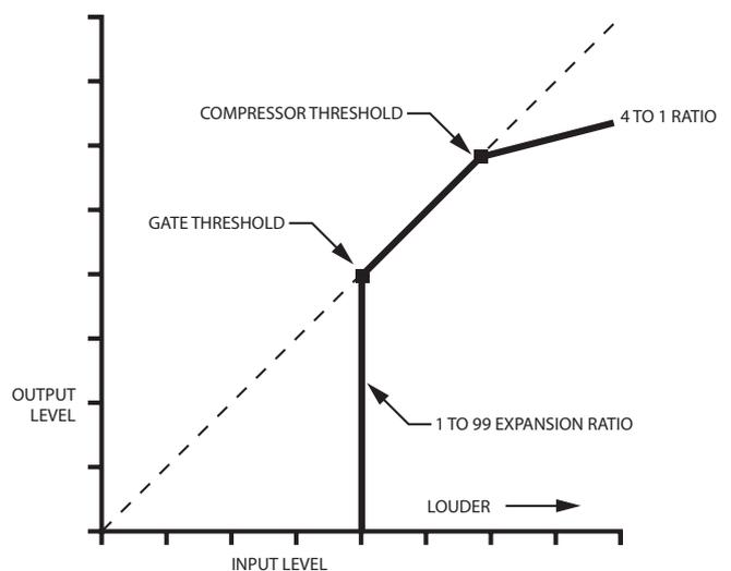
Using this setting, levels above the compressor threshold will be compressed at a 4 to 1 ratio. Levels below the compressor threshold but above the gate threshold will not be changed. Levels below the gate threshold will be gated out completely.
