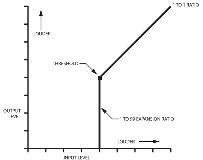
Sounds that are louder than the threshold get “through the gate” unchanged. Sounds that are below the threshold are not heard. Gates can be used to great effect in processing drum tracks where sounds from the other instruments in the drum set leak through the mike of the instrument being recorded. Gates are also used frequently to “gate off” a reverb tail or the ringing from an insufficiently damped drum head.
