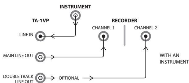
If you are recording directly to a tape deck or hard disk recorder, patch the output from an instrument into the TA-1VP's **LINE IN** and the TA-1VP's **MAIN LINE OUT** into your recorder. If you will be using the TA-1VP's Double Tracking function in stereo mode, patch the TA-1VP's **DOUBLE TRACK LINE OUT** to a separate channel on your recorder.
