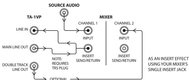
If (as is more common) your mixer has a single insert jack, you will need a "Y" cable with one 1/4" TRS (Tip, Ring,
