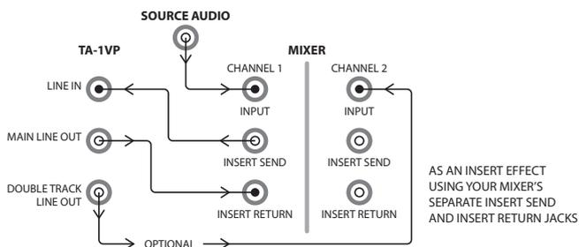
This is probably the most common setup for the TA-1VP. It will function as a pre-fader effect on one of your mixer's input channels.
