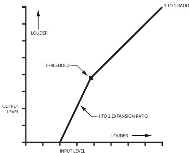
When expanders use ratios higher than 1:10, sounds below the threshold are faded out very rapidly. This effect is called gating and can sound very abrupt. Adjusting the gate ratio can smooth out the abrupt change. The graph below shows the input/output curve for a typical gate.
