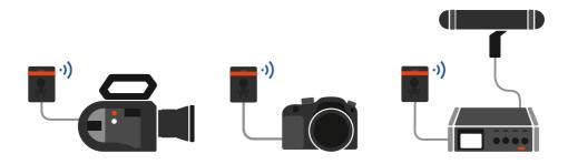
Tentacles can be used with nearly any recording device: Cameras, audio recorders, monitors and more. All they need in order to work with a Tentacle is either a dedicated timecode input or at least one audio channel. There are basically two groups of equipment:
