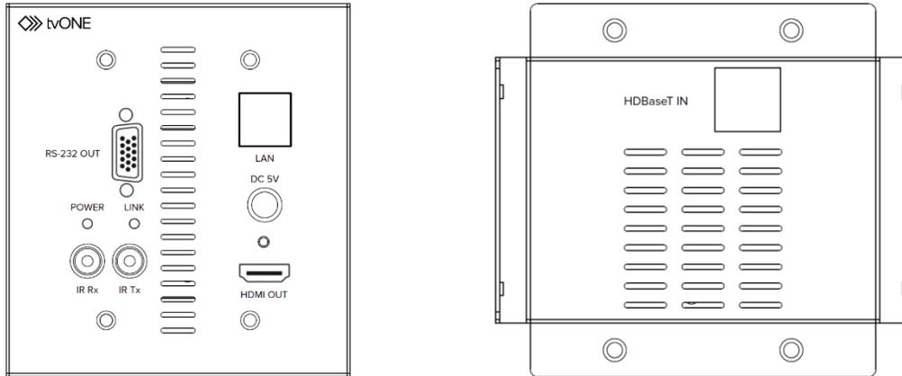
1. At the remote location, connect the Cat.5e/Cat.6 cable to the Receiver's CAT5e/6 In port. Ensure that the RJ45 connector is securely locked into the receiver's port.
