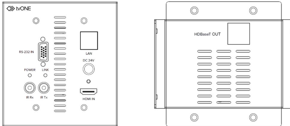
1. Connect the HDMI source device's output to the HDMI IN port of the 1T-CT-653-USWP Transmitter, using an appropriate HDMI cable, (1 Meter (~3') in length for 12 bit signals, 10 meters (~33') for 8 bit signals).
