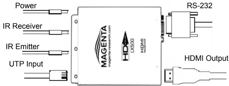
Figure 3-2. Connections on the Receiver
