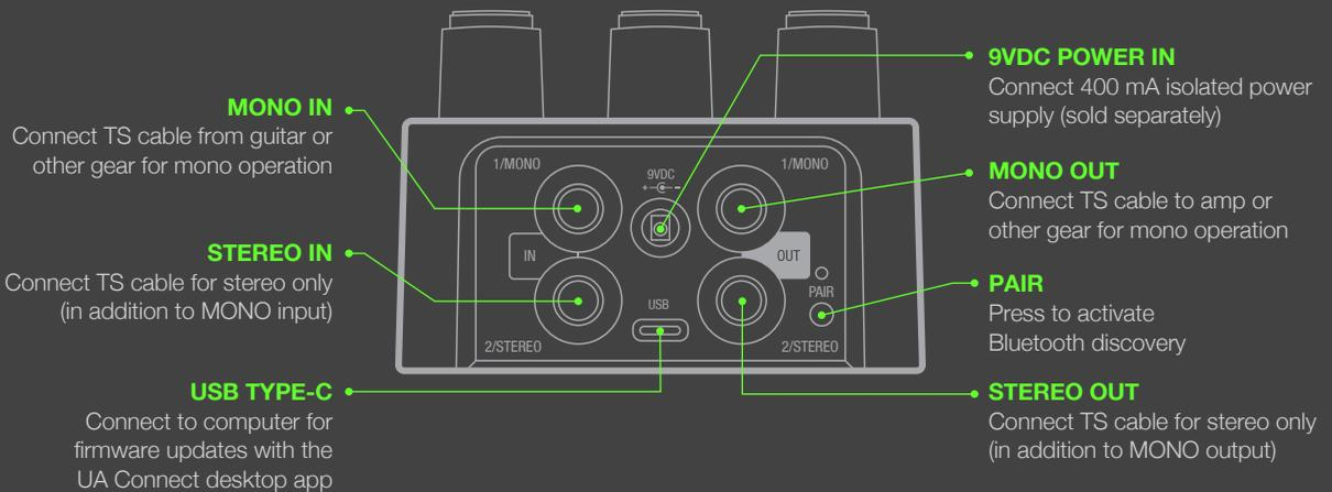
**Power Supply** Isolated 9VDC, center-negative, 400 mA minimum, 2.1x5.5 mm barrel connector (sold separately)
