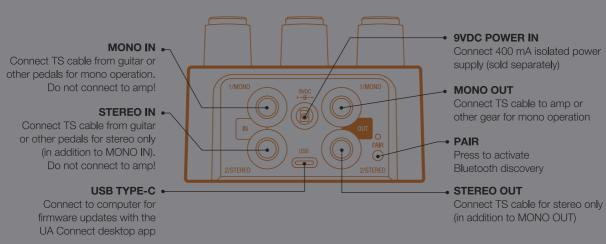
Power Supply Isolated 9VDC, center-negative, 400 mA minimum,
