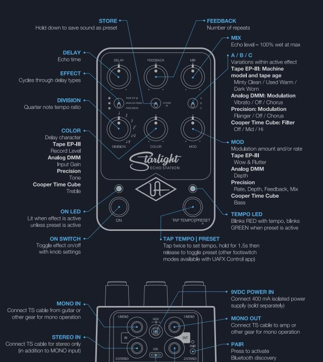
Power Supply Isolated 9VDC, center-negative, 400 mA minimum,
