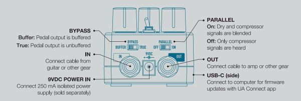
Power Supply Isolated 9VDC, center-negative, 250 mA minimum, 2.1x5.5 mm barrel connector (sold separately)
