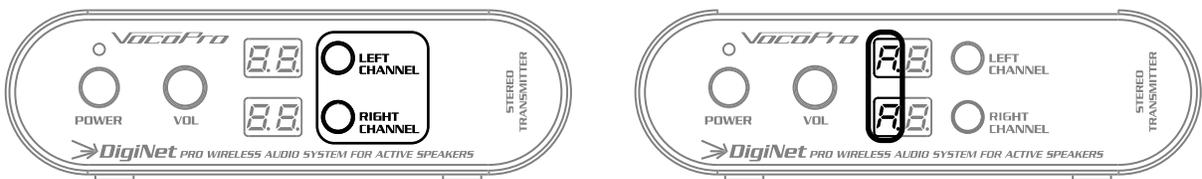
3. Press Left/Right Channel button to toggle through A or B frequency sets
