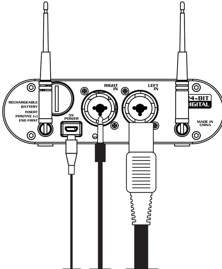
3. Adjust your input source volume and then the transmitter output volume.
