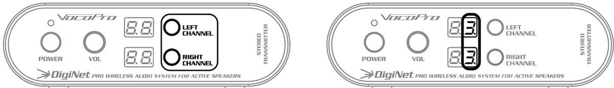
2. Press the Left/Right Channel buttons to increase the transmitting frequency channel number ID
