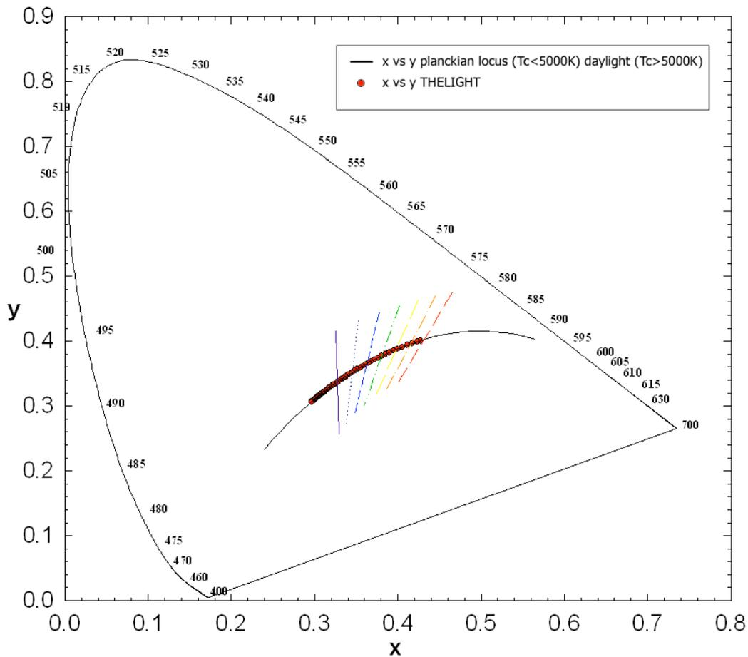
Shown on the diagram are the THELIGHT lamp head chromaticity coordinates [x, y CIE-1931] feed and digitally controlled by its Control Unit and they are compared with the reference illuminants. These reference illuminants are the Planckian locus radiator set below 5000K and the CIE daylight reference is set over 5000K. The Planckian locus radiator references the chromaticity for several tungsten lamps colour temperatures while the daylight locus typify daylight type D illuminants.
