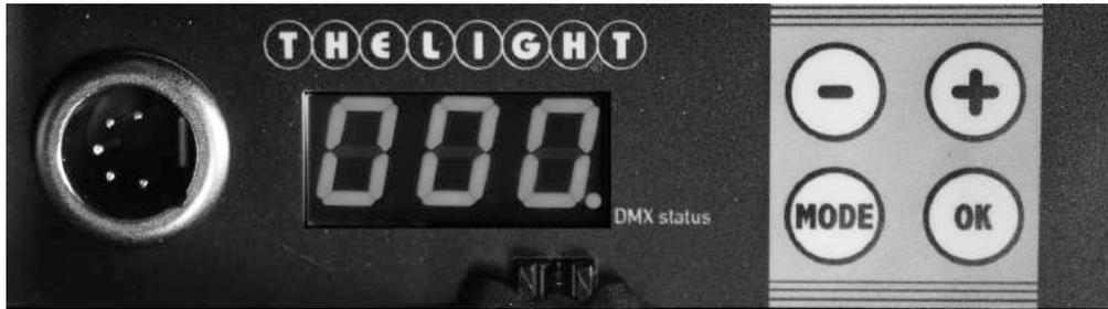
Use DMX XLR-5 in&out splitter cables (ref. THE-VL-DMXinout) to daisy chain several VELVET panels or mix them within any DMX line of different fixtures.
