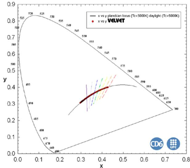
Shown on the diagram are the VELVET lamp head chromaticity coordinates (x, y CIE-1931) feed and digitally controlled by its Control Unit and they are compared with the reference illuminants. These reference illuminants are the Planckian locus radiator set below 5000K and the CIE daylight reference is set over 5000K. The Planckian locus radiator references the chromaticity for several tungsten lamps color temperatures while the daylight locus typify daylight type D illuminants.
