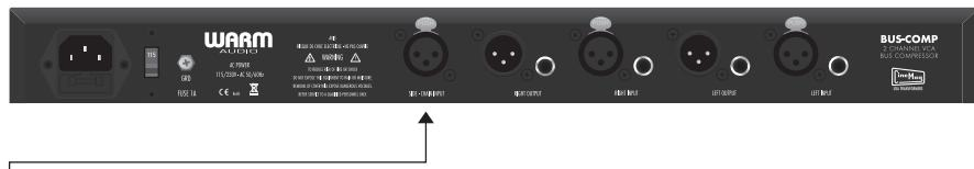
When nothing is plugged into the side-chain input, it is the compressor alone that determines what the audio sounds like as it leaves the compressor. However, if you want to modify the sound before it leaves the compressor, the side-chain input is where you can make that happen.
