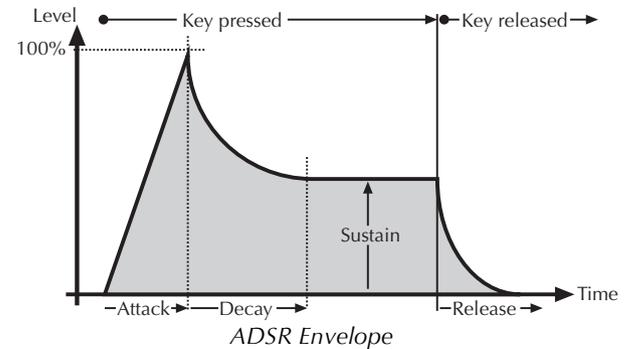
The envelope is started by pressing a key. It ascends to its maximum value at the rate determined by the **Attack** parameter. It then descends at the rate determined by the **Decay** value until it reaches the predetermined **Sustain** value. It remains at this value until the key is released. The envelope then descends to zero at the rate determined by the **Release** parameter.
