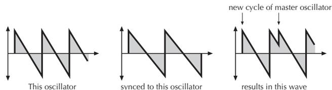
✳ Use **Sync** for Lead or Solo sounds. Set Oscillator 2 to play one octave and 7 semitones higher, apply an envelope to its pitch with positive amount and you get a screaming sync sound.
